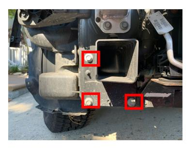
4) You can now install the Frame Extension using the factory 15mm bolts which you just removed AND the 6 grade 8 lock nuts provided. Using a box wrench install the lock nut behind the frame to sandwich it between the nut and the recovery hook mounting plate.
