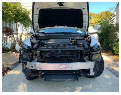
3) Remove the three 15mm bolts holding on the metal brackets on both sides of the vehicle, as well as the 10mm nut on each side.
