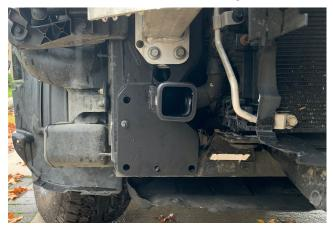
DO NOT torque – Factory aluminum nuts will shear.
